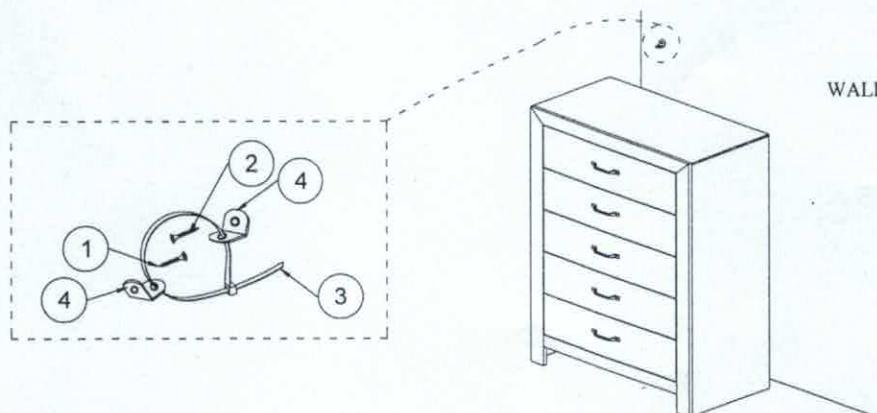
NOTE: MUST TIGHTEN SCREWS PERIODICALLY WITH USE SCREW WILL BECOME LOOSE CHECK TIGHTNESS OF ALL SCREW EVERY 6-8 WEEK. /
